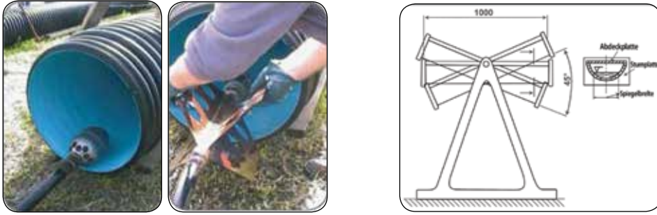
Left: On-Site Testing Left and middle: Abrasion tests using probes. Right: Simulation of Abrasion Test
